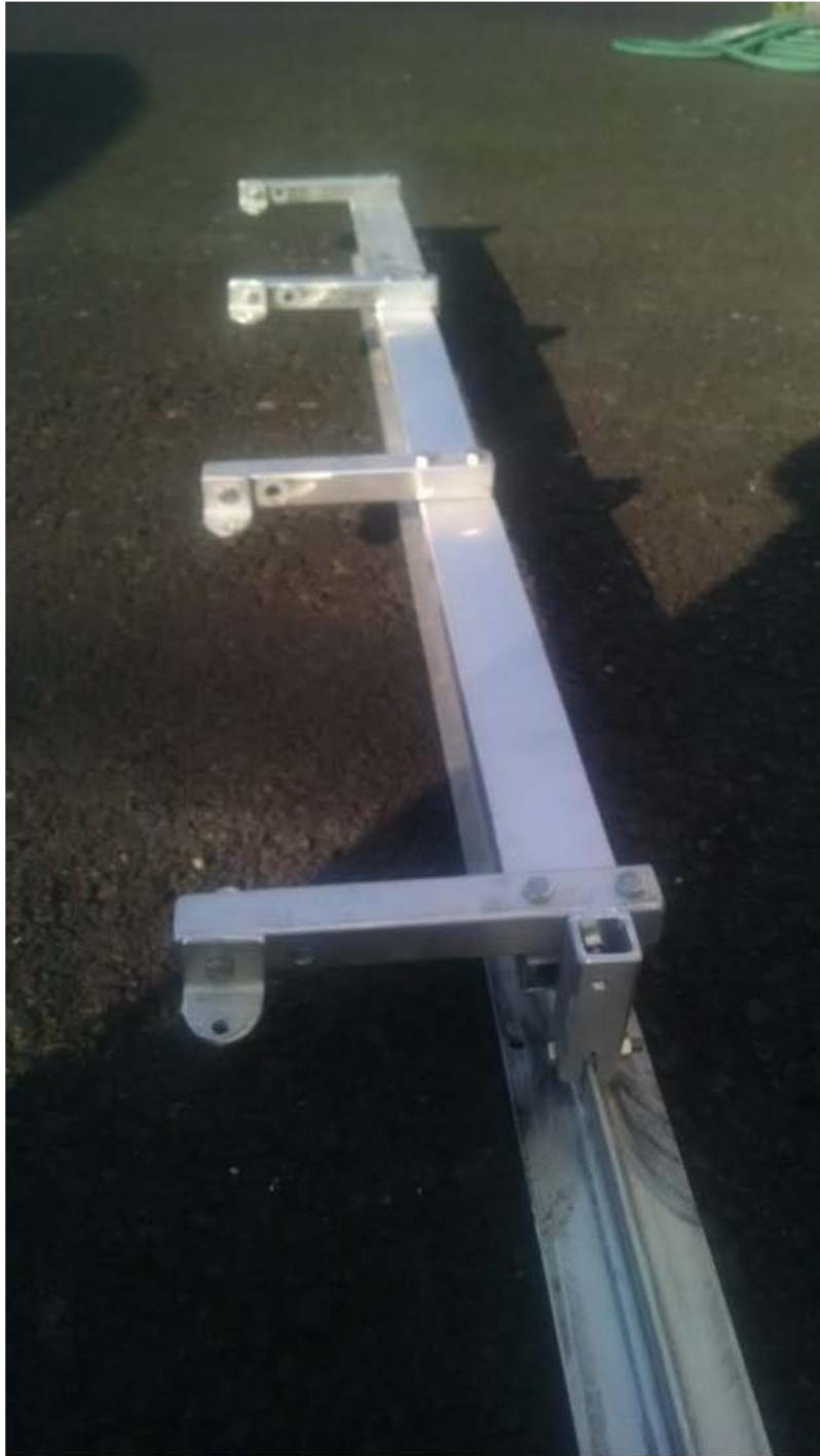
Figure 4. Modified I-beam with two light mounts and two camera mounts to be used in the proposed monitoring. Edges will be rounded prior to deployment.
