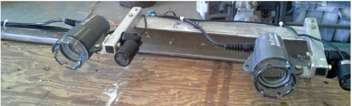
Figure 3. Cameras and IR lights mounted to a modified I-beam trolley as used in the July 2014 deployments. The upper I-beam flange has been removed (except where instruments are mounted). The web has also been largely removed, and serves as a cable guide (left hand portion of lower photo). The lower flange rides inside the mounting channel (upper photo). Edges have been rounded and bolts will be covered in silicone prior to deployment. For reference, the Sea View IR light sources measure 4.5" diameter X 7.25" long.
